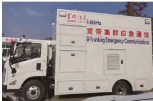
Capinfo's emergency communication vehicle for the 1.4g broadband cluster private network
